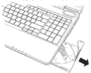
Figure 4-3 Pulling the disc tray open
